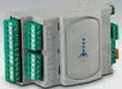
KRS485 - RS485 Serial interface board
